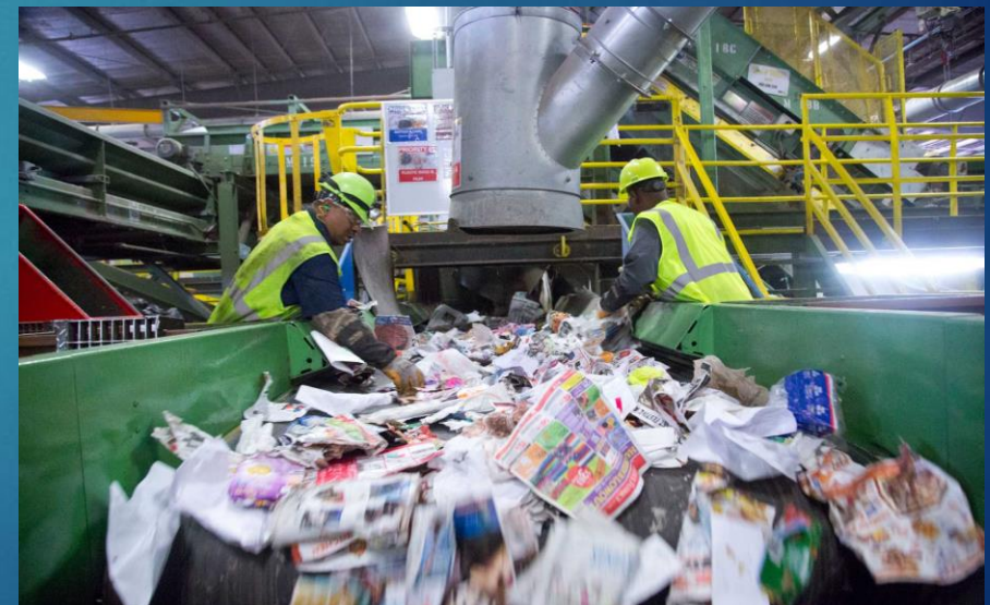
MRF designs incorporates both manual and mechanical separation
