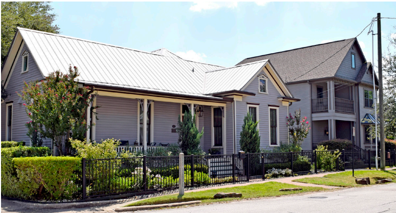
Site design considers street frontage, building setbacks, parking, signage, service and utilities, fencing and screen walls. Shallow front yards, continuous planting strip, and fences are site features noted in this image.
