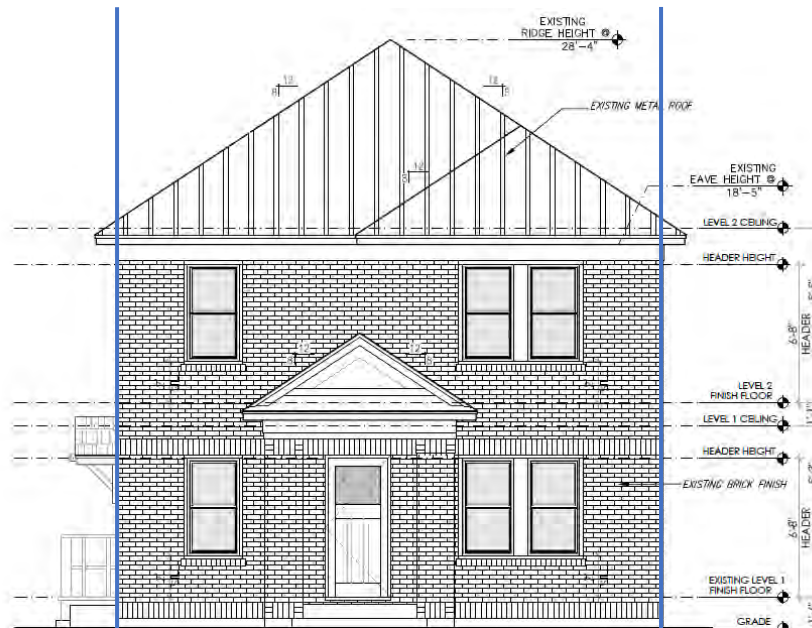
EXISTING HOUSE WEST ELEVATION
