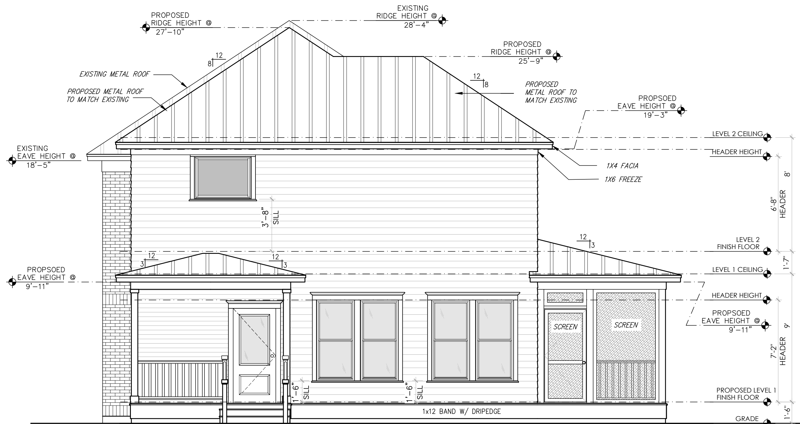
PROPSOED HOUSE EAST ELEVATION Scale: 1/4"= 1'-0"
