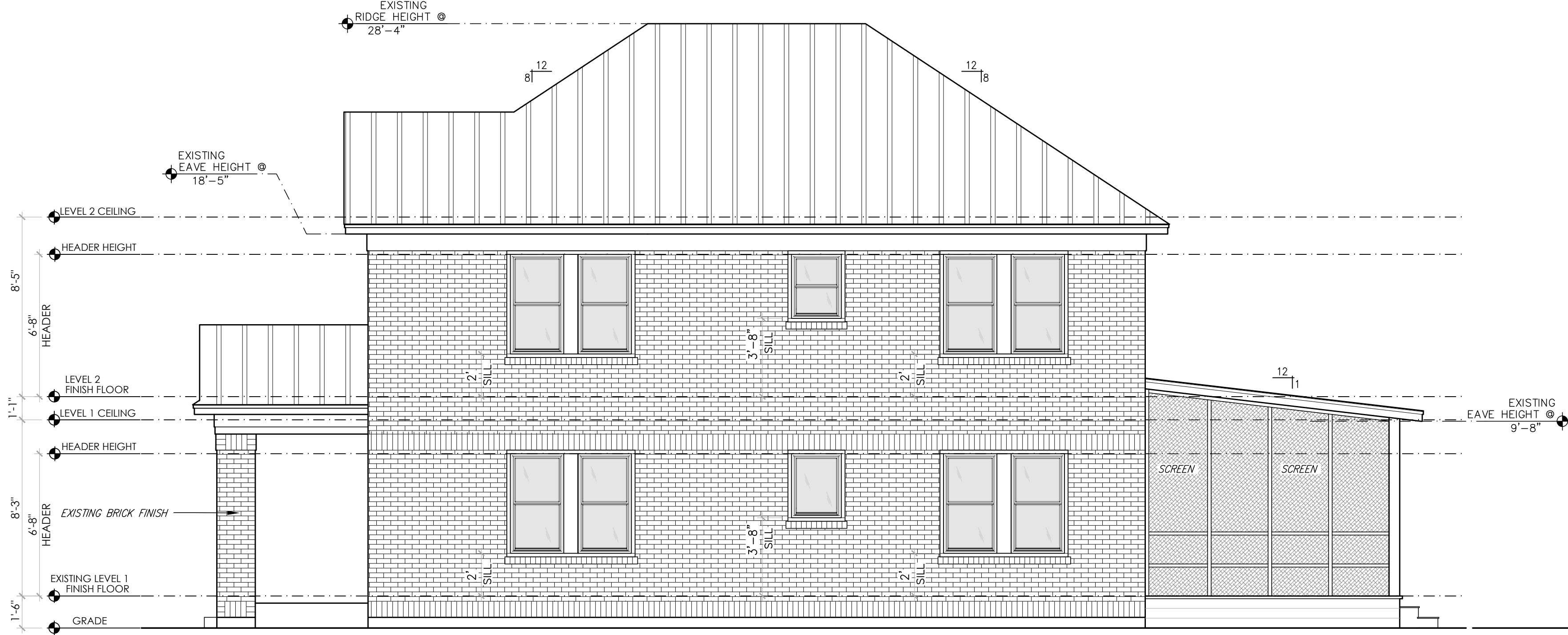
EXISTING HOUSE SOUTH ELEVATION Scale: 1/4"= 1'-0"
