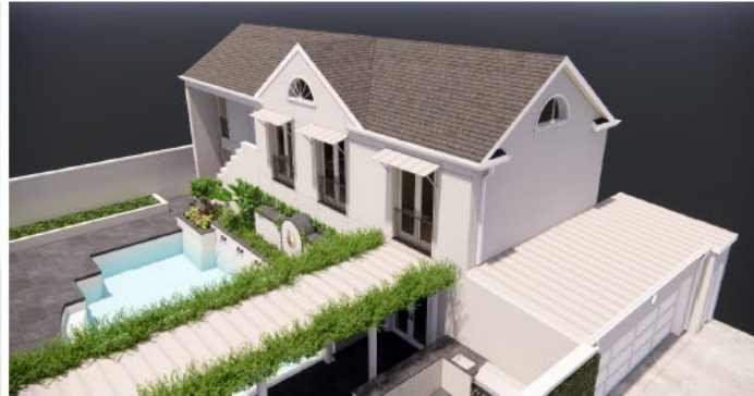
RENDERING OF PROPOSED SHADE AWNINGS AS VIEWED FROM DUNLAVY ST. STYLE & CONSTRUCTION TO MATCH THE COVERED WALKWAY DESIGN. NEW BALCONY RAILING TO MATCH FRONT & REAR ADDITION RAILING DESIGN FOR A CONSISTENT APPEARANCE.
