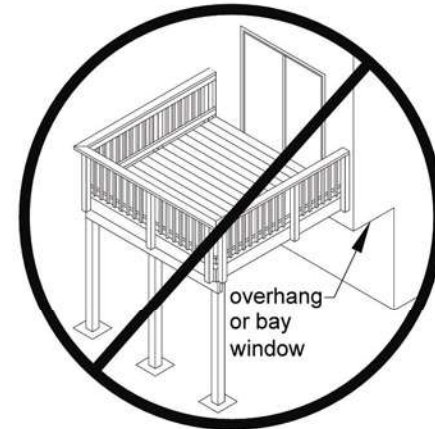
Figure 18. No Attachment to House Overhang
