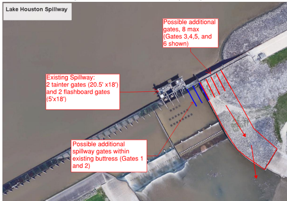
Figure 2: Possible Additional Spillway Gates
